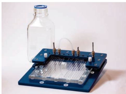
Figure 5. Parallel multilayered microstructured reactor. Internal volume: 9.6 mL.
