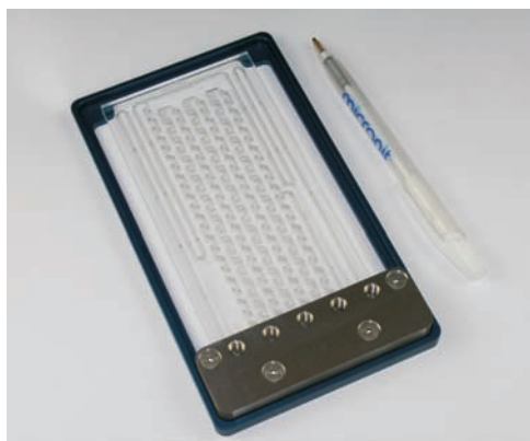
Figure 4. Microstructured flow reactor. Internal volume: 2.4 mL.
